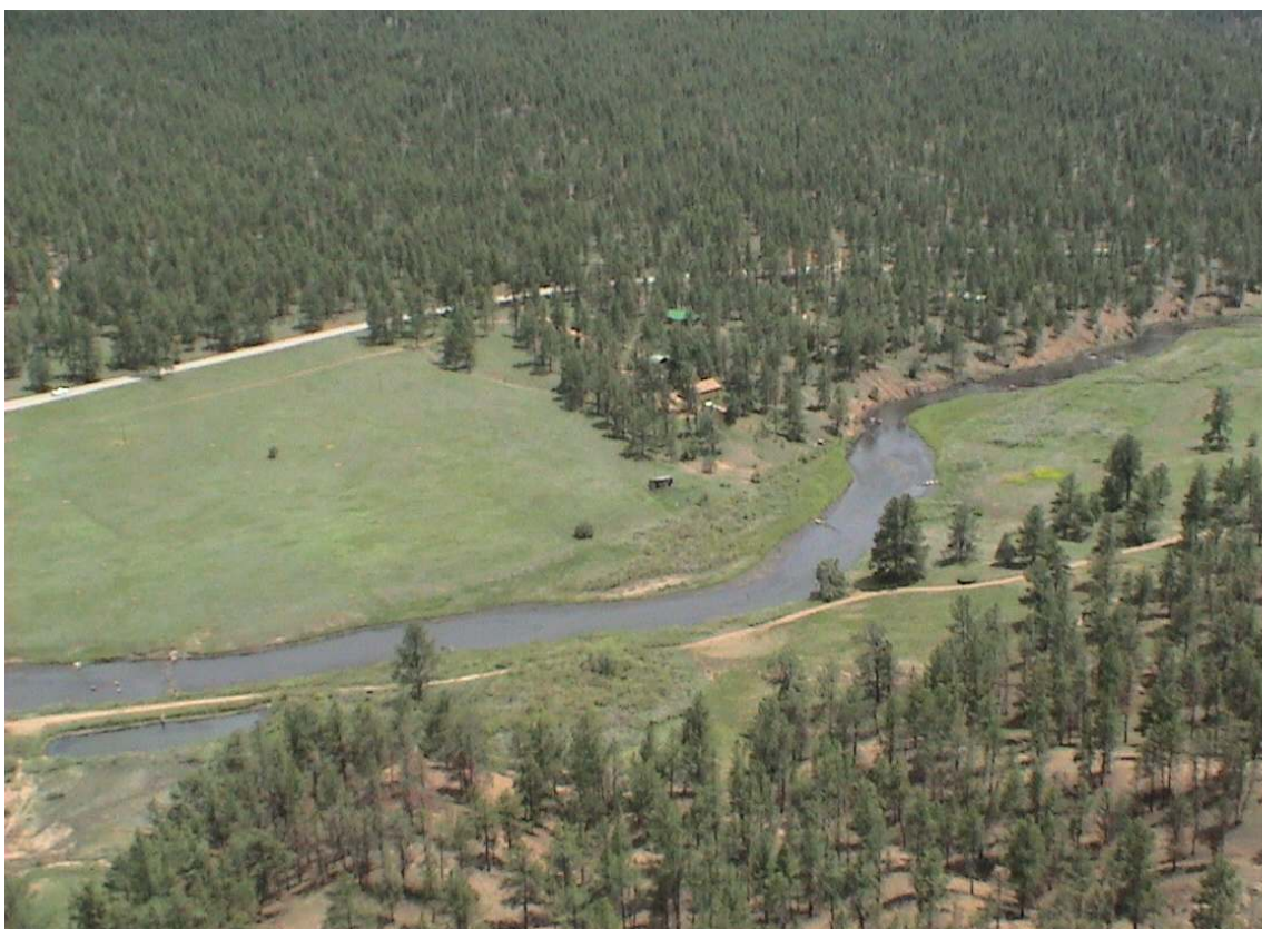
Photo 30: River over-widening due to miss-aligned boulder vanes. Swayback Ranch, CO
