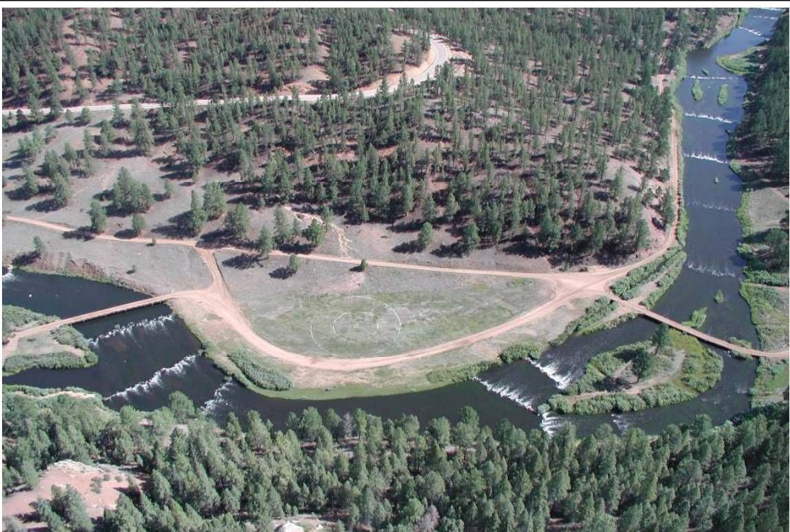
Photo 27: Example of river over-widening due to poorly configured drop structures. Wigwam Club, CO
